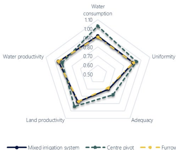
Figure 3. Summary of the performance indicators averaged over five seasons by irrigation method. The five indicators in the figure are normalized using their maximum (100%) or target values. Thus the indicators show extremely low performance at 0 and high performance at 1. For water consumption, a value greater than 1 indicates over consumption.
