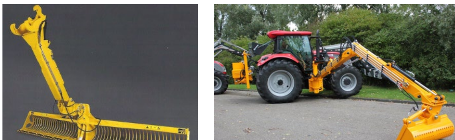
Figure 2-2: New generation, wide (5.5 m) effective buckets currently being produced by the Netherlands private company Herder that was active in the Gezira Scheme back in the 1990s. The MoIWR has re-engaged with Herder to explore collaboration opportunities (Credit: MetaMeta, 2019)
