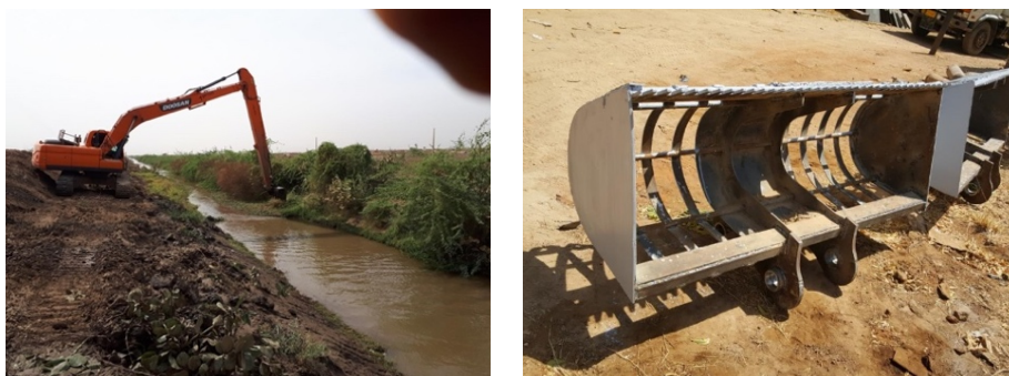
Figure 2-1: Small (1.8 m wide), heavy and ineffective buckets in use by the local private sector in Gezira Scheme (Credit: MetaMeta, 2019)
